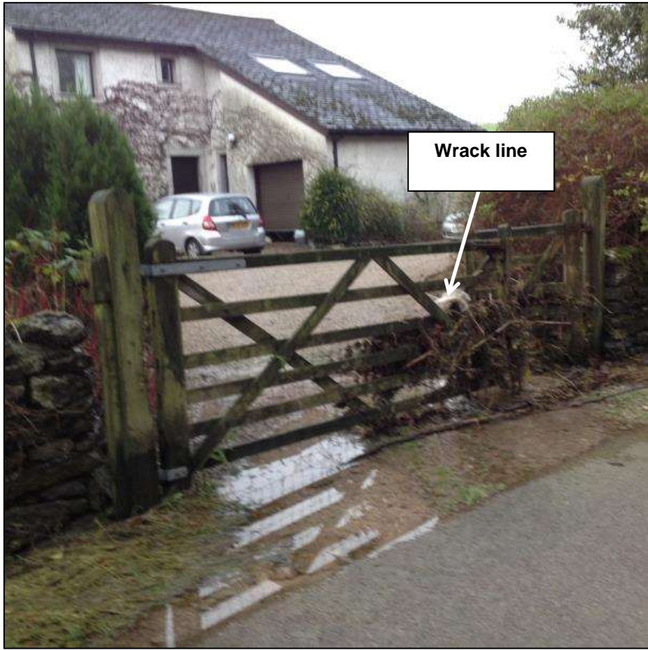
Figure 3: Wrack in an access gate outside properties on the left bank of the River Bela
