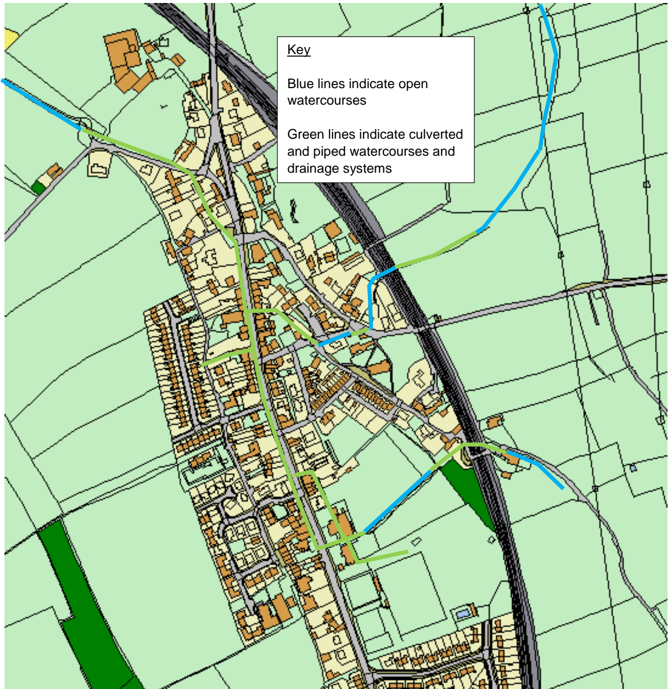
Figure 6: Plan indicating extent of culverted watercourses and drainage systems in the north and central area of Shap.
