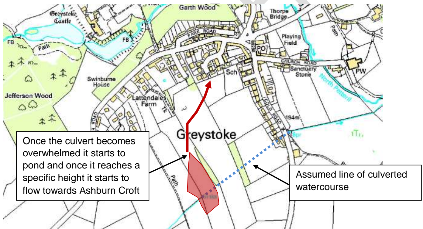
Figure 10: Location of culvert in fields south of Ashburn Croft
