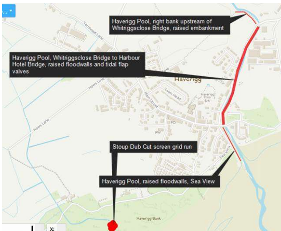
Figure 20: Assets maintained by EA in Haverigg
