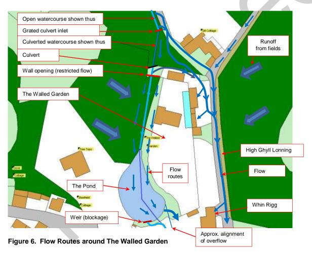
Beyond the downstream end of the blocked culvert, the watercourse encounters The Walled Garden, which has an opening to allow normal flows. However, due to the volume of water on the day part of the flow diverted along the wall to the eastern corner of the property, flooding out buildings and then joining High Ghyll Lonning. These flows then flooded the garage of Whin Rigg on the way down to The Square.
