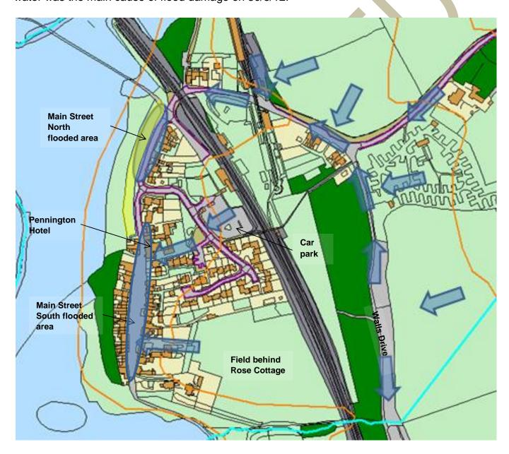
Figure 4. Surface water flow routes (arrows) and main flooded areas (oval). Some water was held back by a sea defence embankment (yellow). Key locations named in the report are identified.
