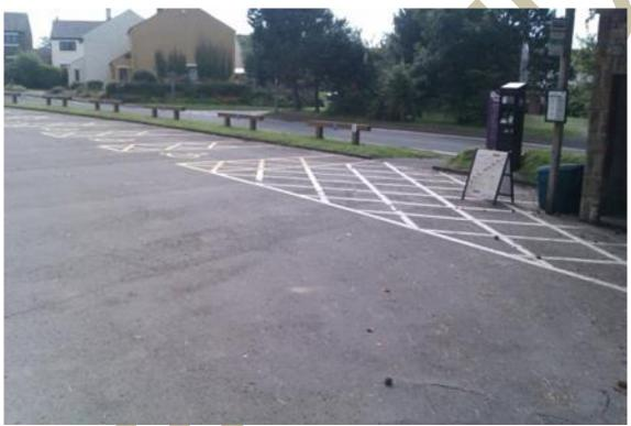
Figure 6. Impermeable surface of the car park and the dropped kerb which provided a flow route for flood water.
