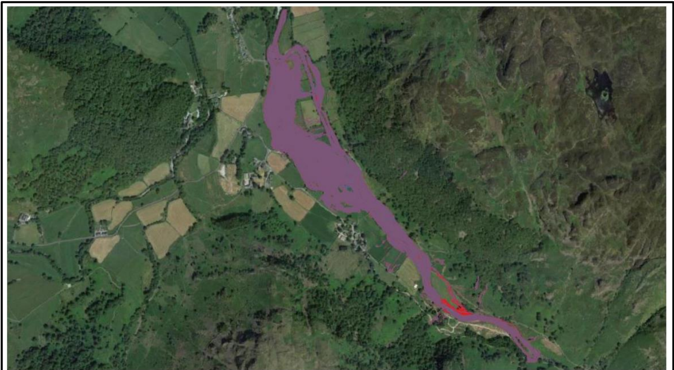
Figure 2.7 1 in 2yr flood extent change, blue = baseline, red = restored (where red is visible indicates flood extent increase, purple indicates no change and blue indicates reduction in flood extent).
