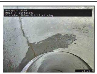
5, 00:02:16, 28.22 m Crack, longitudinal at 8 o'clock
