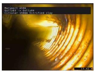
1, 00:02:19, 13.51 m Deformed sewer or drain, 45%
