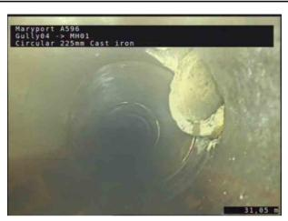
1, 00:02:42, 31.05 m Connection defective, connecting pipe is intruding at 2 o'clock, 100mm dia, intrusion: 15%
