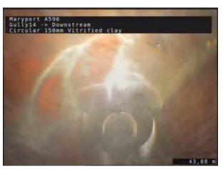
6, 00:04:48, 43.88 m Fractures, multiple from 12 o'clock to 12 o'clock
