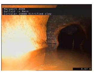
$4,\,00:\!01:\!10,\,6.67$  m Hole in drain or sewer from 12 o'clock to 12 o'clock, Large void
