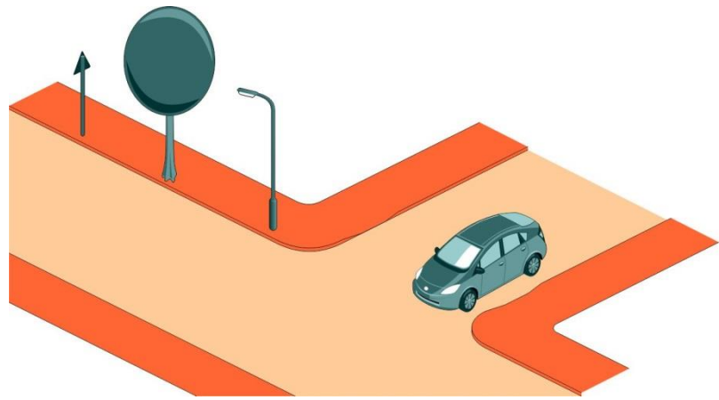
Figure V10: visual obstructions at junctions
