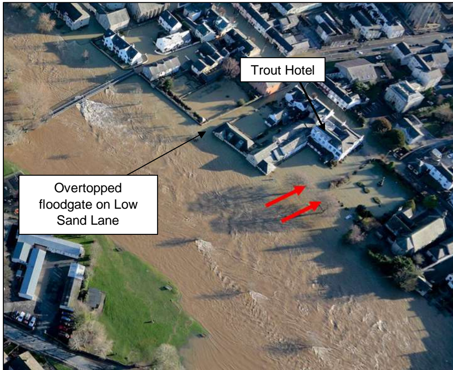
Photograph 3: River Derwent at Main Street area highlighting flow route through the Trout Hotel car park. Photograph provided by Peter Smith Photography. Taken 06/12/2015 12:37
