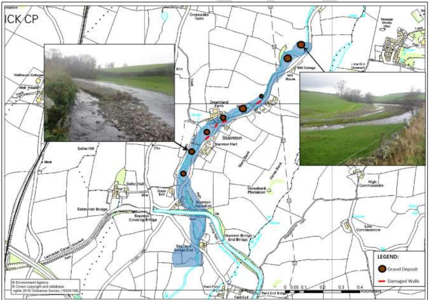
Figure 10 – Location of gravel deposits and damaged highway walls
