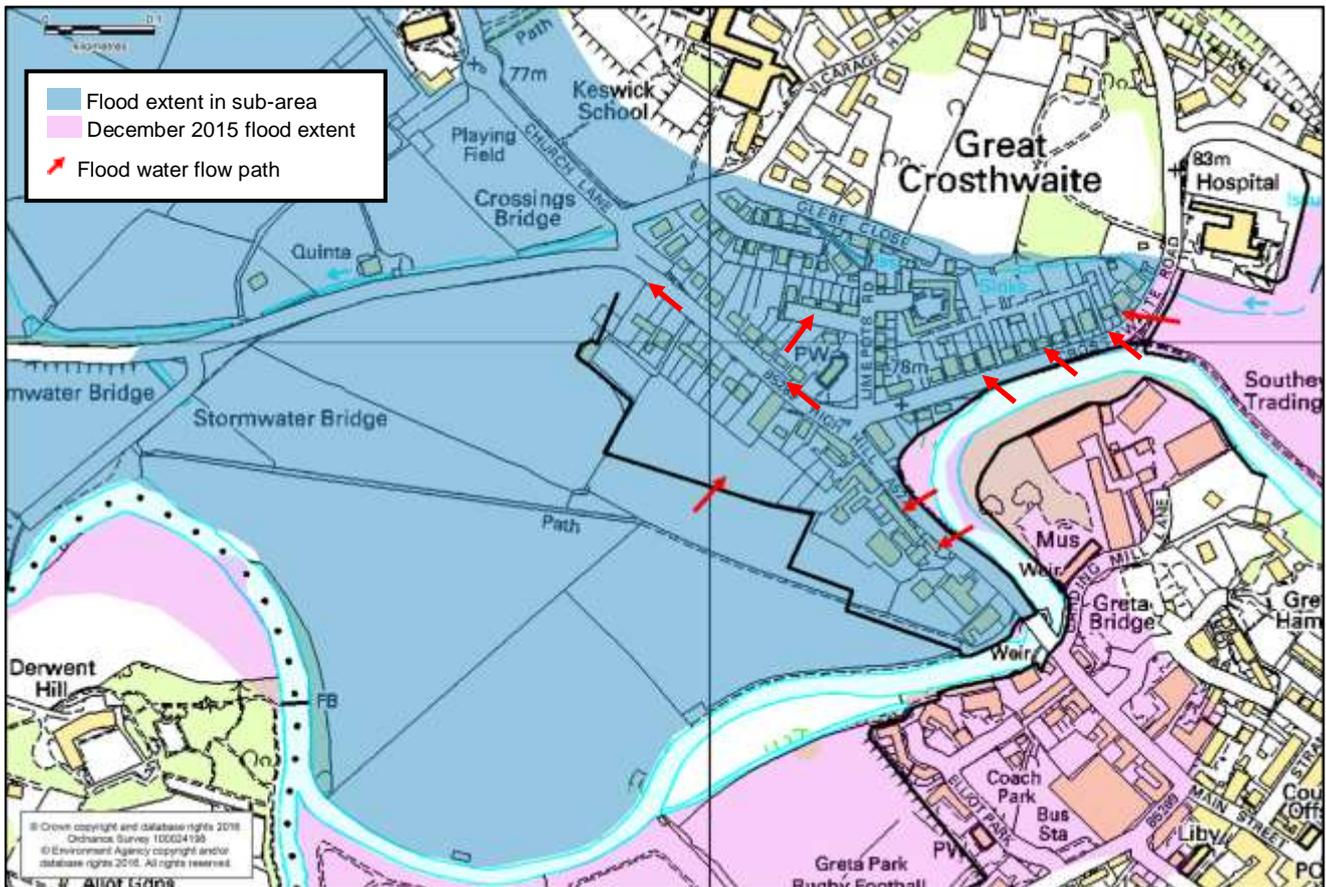
**Figure 22: Source of Flooding and Flood Extent at High Hill**
