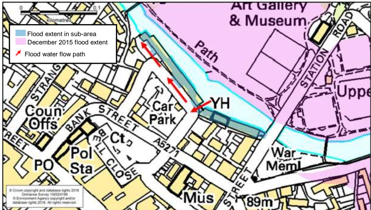
**Figure 19: Source of flooding and Flood Extent at Greta Side**
