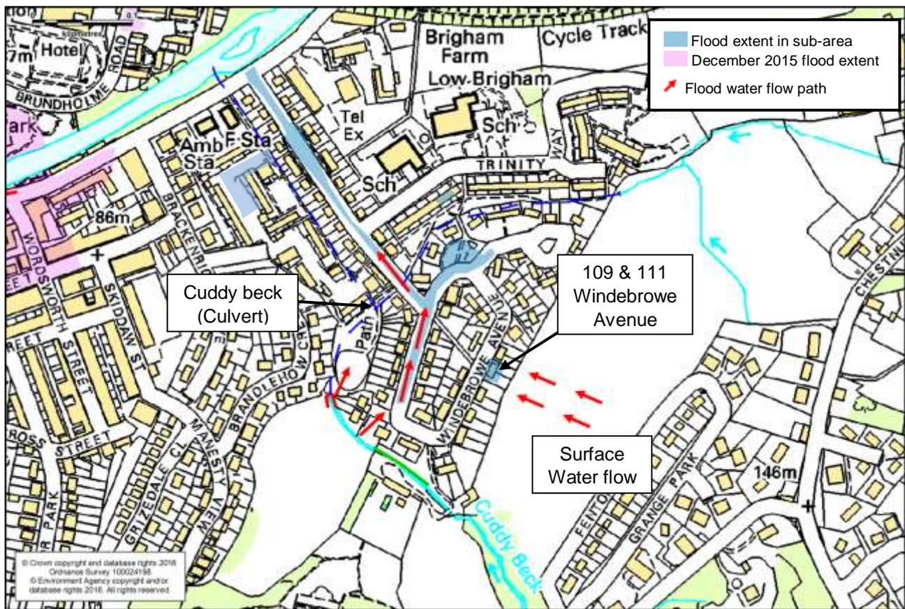
**Figure 15: Source of flooding and flood extent at Windebrowe Avenue and Trinity Way**
