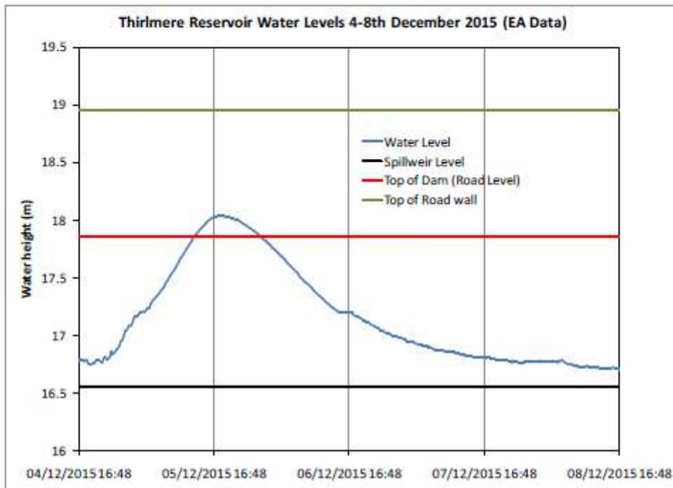
**Figure 7: Environment Agency water level data for Thirlmere showing how the level was higher than the dam road level during Storm Desmond.**
