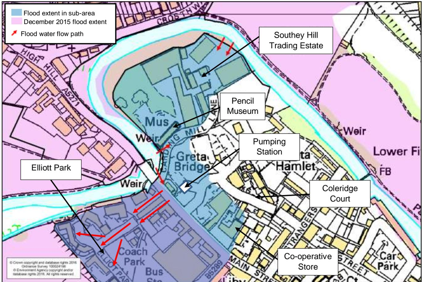
**Figure 20: Source of Flooding and Flood Extent at North of Main Street – Southey Hill Trading Estate/area**
