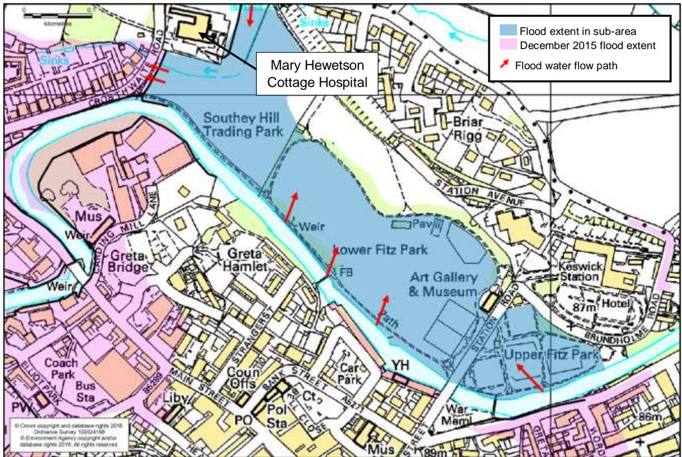
**Figure 18: Source of flooding and Flood Extent map at Upper and Lower Fitz Park**
