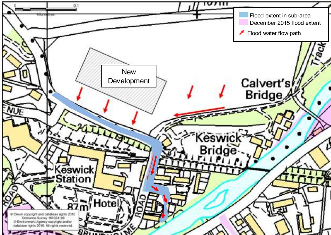
Figure 16: Source of flooding and Flood Extent at Brundholme Road
