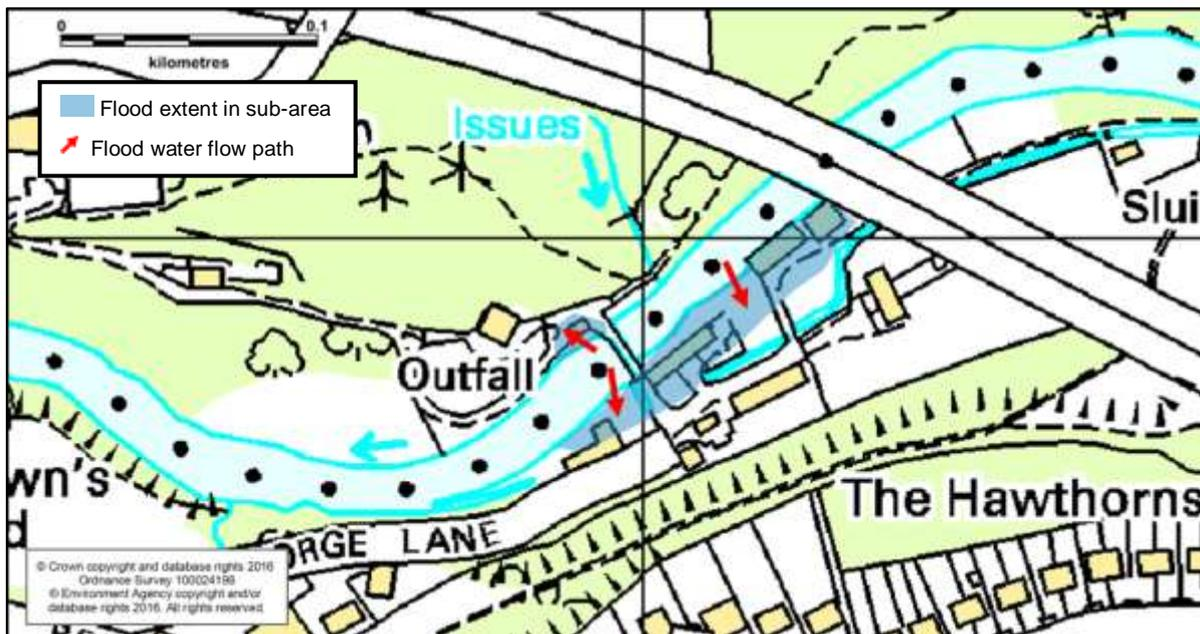
**Figure 13: Source of Flooding and Flood extent at Forge Bridge area**
