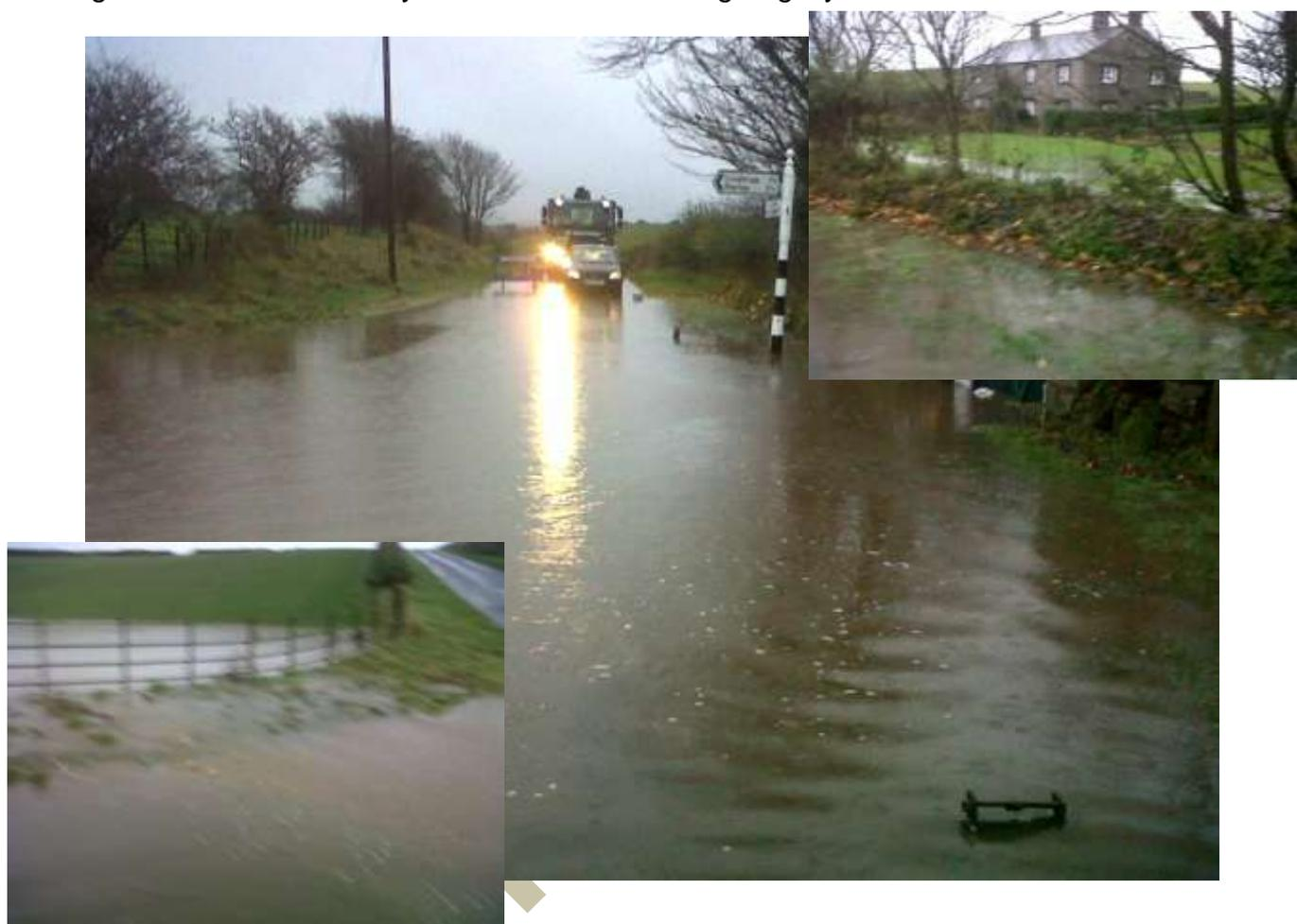
**Figure 5. Flood water flowing out of the corner of the field (bottom inset) and flooding the road where a dislodged gully grating shows above the water. Flood water had not reached the house (top inset). Photos taken 22/11/12.**
